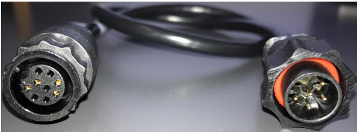
000-13977-001 Adapter cable. Note that pin 9 on the female connector is populated for XID.
